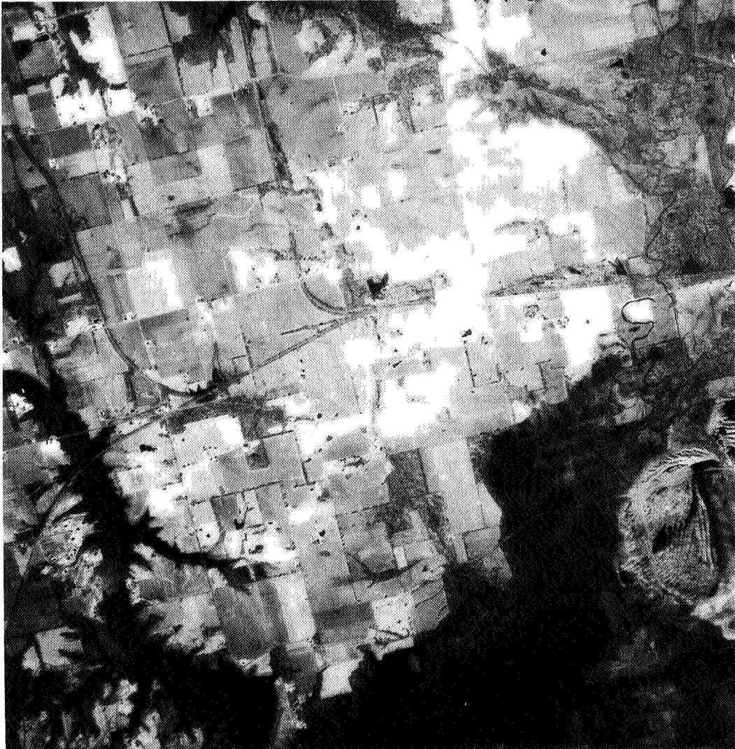
Figure 5. Black and white infrared image of part of Sullivan County, Indiana, showing extensive surface subsidence along Busseron Creek caused by underground coal mining.
