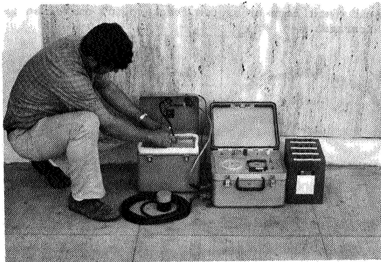
Figure 3: Satellite transmitter (left), seismic sensor (left foreground), seismic event counter (center), and batteries (right) used to monitor seismic activity and send the data to the satellite.
