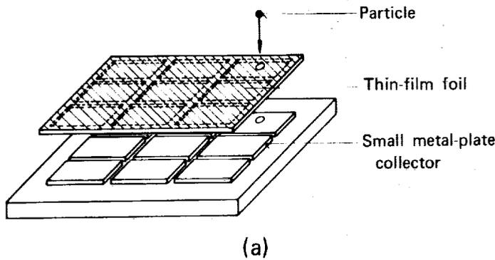
FIGURE 5.—(a) Controlled collector by hole identification.
