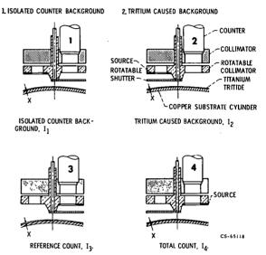
for each thickness measurement. A fourth count, obtained with the monitor configuration 1 in the figure, is the isolated counter background count. This count,  $I_1$ , is independent of the radioactive cadmium source or the tritium film, and, therefore, this measurement is not necessary for every thickness determination.
