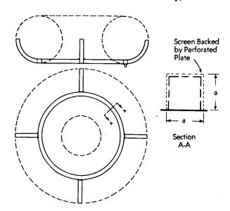
munication channels act as baffles and tend to maintain uniform propellant distribution in the tank when spacecraft spin rates are increased or decreased. Thus, in addition to providing gas-free propellant, the device controls propellant distribution and movement within the tank, and minimizes the requirements placed on the spacecraft attitude-control system.
