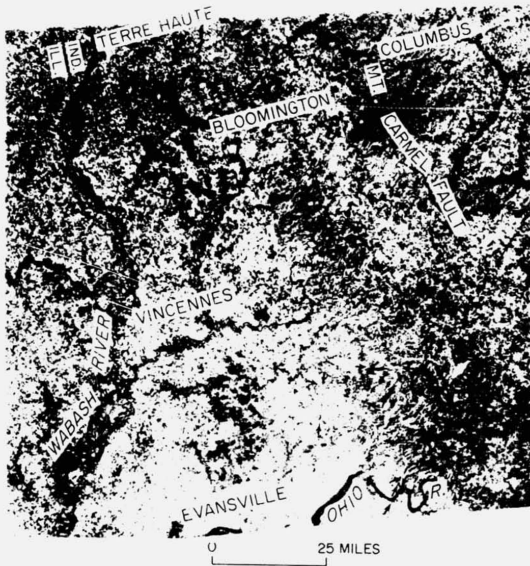
Figure 2. ERTS-1 image (1105-15595-7, 5 November 72) of southwestern Indiana, showing fracture patterns along drainageways and ridges in upland areas underlain by Mississippian limestone and siltstone.
