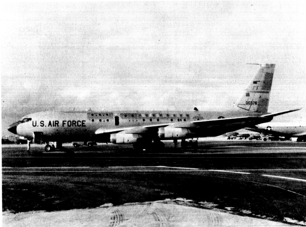
Figure 1. KC-135 with blade antenna for satellite communication.
