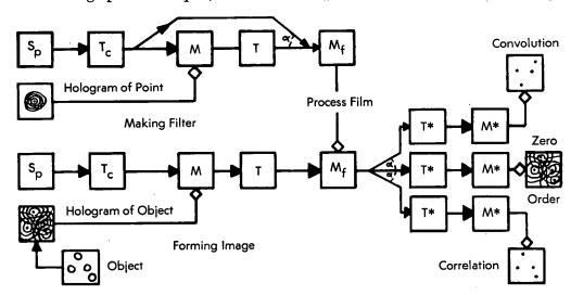
reference beam causes the image to be offset from the DC term. Microwave holograms are made without an offset reference beam, but it has been found that a Vander Lugt filter can be used to produce the image offset. Also, the filter permits "decoding" of holograms in contrast with the usual practice of reconstructing visible-light analogs of the original microwave wavefronts.
