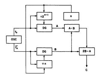
The A-B and 2B-A circuits are identical and very simple, as shown in the schematic diagram. A flip-flop is set and reset on A pulses and B pulses, respectively. If two B pulses occur within the period between two A pulses, an output pulse is registered.
