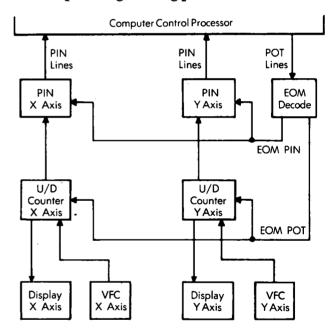
Hz in two ranges. The pulses from the VFC oscillator and controller are counted in an up/down (U/D)counter having a count display which shows the decimal count and the direction of counting. Counts cycle to 999 in the positive direction, change sign and then count from -998 to zero; the counting and display is cyclic. It is necessary only to keep track of the number of cycles in a large displacement; the three decimal digits in the positive and negative directions
