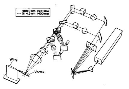
Laser Doppler velocimeters are especially useful for the measurement of localized fluid velocities when perturbation of the flowfield is not desired. The basic principle of operation is that coherent laser light scattered from particulate matter in a fluid moving with a given velocity is Doppler-shifted by an amount dependent upon the laser wavelength in a vacuum, the index of refraction of the scattering medium, and unit vectors in the directions of the scattered and incident waves.
