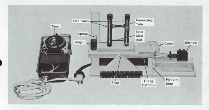
A device for automatically transferring a known volume of bacterial culture from one test tube to another, under sterile conditions, is now being used at Langley Research Center. It can perform such a transfer without human involvement, during non-working hours, as overnight or on weekends.
