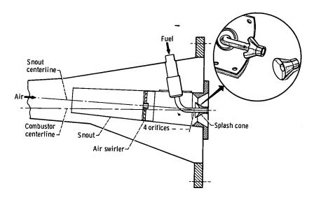
An air-atomizing fuel nozzle has been developed which utilizes the momentum of the inlet-air to atomize and distribute the fuel to improve burning characteristics and reduce pollutant emissions of turbojet engines. Tests have shown that emissions of nitric-oxide, carbon monoxide, and unburned hydrocarbons were significantly reduced with the splash-cone fuel nozzle when compared with those produced with conventional pressure-atomizing fuel nozzles.
