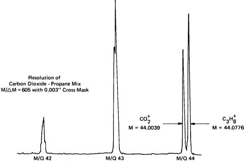
**Resolution in Quadrupole Mass Spectrometer**
