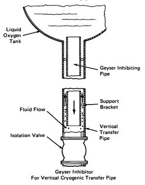
The pipe system as shown in the illustration comprises a smaller concentric pipe welded to the main pipe. The inner pipe begins above the bottom of an isolation valve and terminates in the storage tank at the top.
