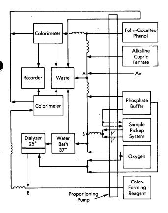
dinarily used for automated analyses can readily be modified to accommodate the analytical scheme shown in the flow diagram. Unlike prior semiautomated methods, the newly developed system includes steps and devices for mixing the drug with enzyme and cofactor in the presence of pure oxygen, dialyzing the resulting metabolite against buffer, and determining the amount of metabolite by a colorimetric method.
