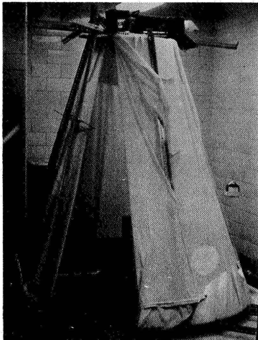
FIGURE 2. Slide projector used as light source is mounted on top of framework. Rotating table and pigeon's box can be seen through folded-back sheet which zipped closed when the birds were working. Small arrow points to last mirror in the series, which could be moved up and down the track on which it is mounted to change the altitude of the light.
