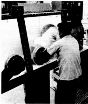
Figure 8.--Transferring the Bags of LiH into the N 2 Atmosphere Box
