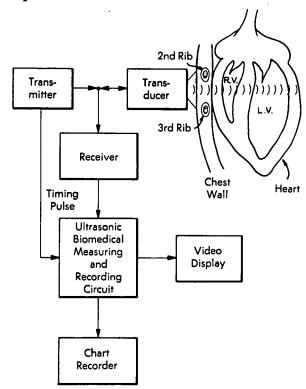
and positioned to direct its beam of ultrasonic wave energy into the portion of the body under observation, for example, the heart of a patient with a cardiac ailment. An ultrasonic transmitter energizes the transducer with a train of pulsed energy, typically 2.25 MHz with pulse duration of one to several microseconds
