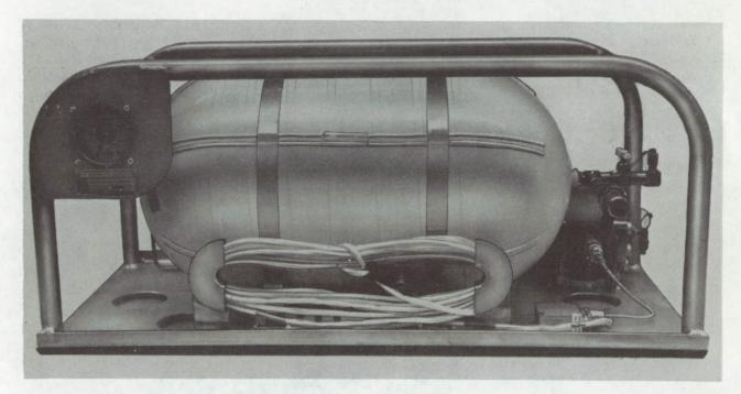
A leak test system used for quantitative determination of leak rates in large pressurized compartments in an aerospace program appears feasible for adaptation in industrial fabrication and maintenance operations.
