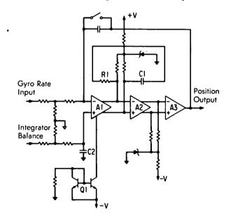
flight-qualified components. The system employs a pair of transistors in a differential input stage which is an integral part of a temperature-controlled semiconductor substrate.
