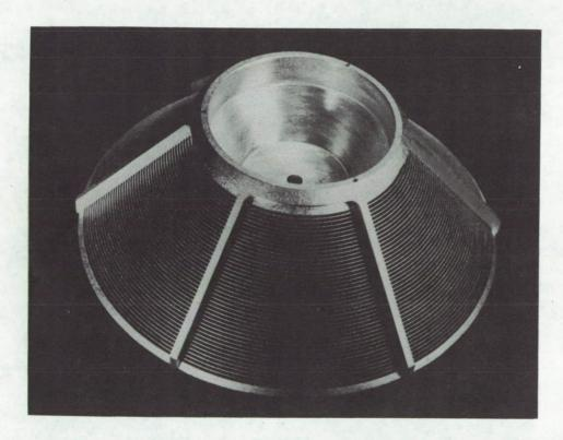
A high-vacuum diffusion pump baffle, positioned immediately above the pump stack, prevents vaporized pumping oil from entering and contaminating the test chamber. The baffle (see figure) consists of a series of concentric rings between the top of the diffusion pump stack and the vacuum pump wall. The pumping vapor is collected and condensed on the baffle and flows back to the pump base along four rods. Although the baffle has no provisions for cooling, test results indicate a
