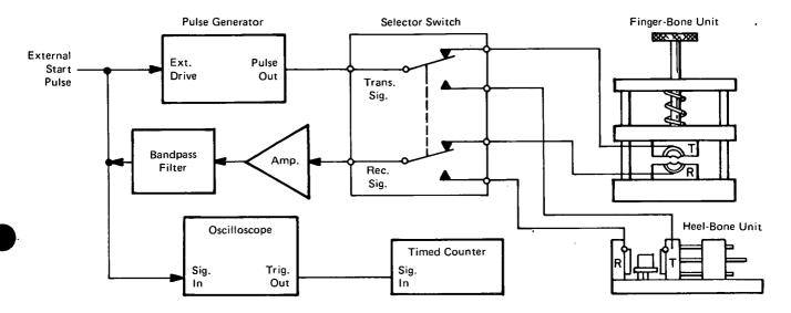
Changes in the density of human bones can be rapidly and accurately determined by an ultrasonic device that was originally developed for in-flight testing of astronauts' bones during extended space missions. Comparable in size, weight, and power consumption to a portable television set, the device may also be used in hospitals for monitoring the skeletal condition of patients immobilized for long periods.
