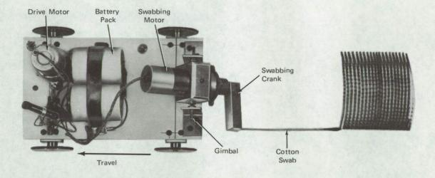
The Mobile Surface Sampling Cart, as shown in the figure, is a device which automatically swabs surfaces for the recovery of microorganisms; it operates without human involvement and provides for control of swabbing speed, rotation of the cotton swab, and the pressure and angle applied to the swab.
