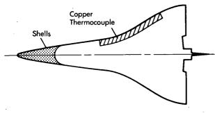
on thin-skinned surfaces in order to obtain accurate measurements. Construction of structurally rigid and accurately duplicated models which have thin skins at measurement points by conventional model-shop techniques is difficult and expensive. The improved technique described below makes possible the fabrication of inexpensive wind tunnel models which have thin-skin shells and thermocouples at specific areas on their surfaces.
