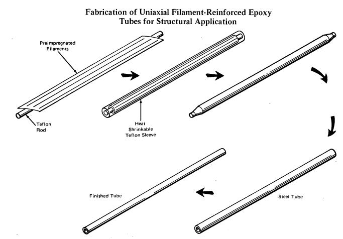
The high strength, high stiffness, and low density of filament-reinforced composite materials have stimulated considerable interest in their potential application to aerospace structures. During the course of research on composite materials, a unique process was developed for fabricating uniaxial filament-reinforced epoxy tubes of suitable quality for structural application.
