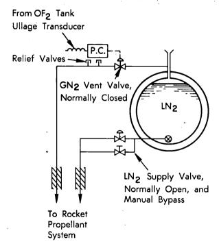
in the  $OF_2$  tank as the liquid temperature and vapor pressure of the  $OF_2$  rises or falls. The vent valve cycles slowly between an open and closed position to maintain  $OF_2$  temperature somewhat above or below the setpoint.
