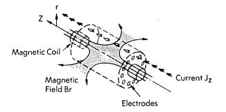
velocity of the rotating mixture must be supersonic. When the gas mixture consists of very light components (such as hydrogen and deuterium) or heavy components at high temperature, the speed of sound in the gas mixture is so large that mechanical rotation becomes impractical; the required rotational velocity is so large that centrifugal forces exceed the structural limits of the mechanism used to rotate the mixture.
