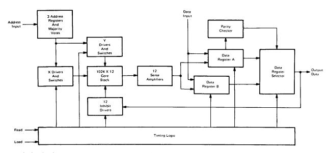
A dual redundant core memory system prevents loss of memory data when a single drive circuit failure occurs. The system requires two address locations and a parity bit for each word. It incorporates series redundant drive switch circuits, triple redundant majority voted memory timing functions, and two data registers to provide functional dual redundancy. The signal flow through these circuits is shown in the figure.
