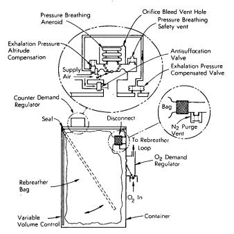
The counter-lung is a flexible bag within a rigid container. The inside of the bag is connected to the breathing loop; the outside is pressurized with air at about one inch of water pressure above cabin pressure to prevent cabin air from leaking into the system. At altitudes where the rebreathing loop must be operated at pressures over ambient, the counter-lung is pressurized to the standard breathing schedule starting at 11.6 km cabin altitude.
