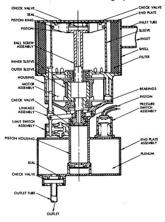
The check valves are supported by flat flexure plates with essentially zero, static spring loads. Piston movement actuates the check valves by utilization of the inherent forces developed by differential pressure and inertia. The low cracking pressure (virtually zero) is important for proper operation of the first-stage suction stroke because of the low ambient pressure differential available at the pump inlet.
