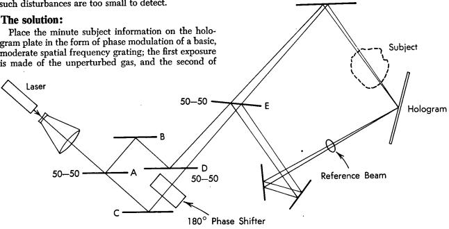
the gas in the perturbed state. Since the system responds only to changes in the subject between exposures, perfect optics are not required. The readout resembles that from a double exposure, subfringe, holographic interferogram, that is, the subject perturbations show up as brightenings on a dark background.
