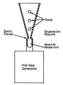
Previous forms of gasdynamic lasers have relied on population inversions created among the lower vibrational levels of a polyatomic gas, such as carbon dioxide. Because such lasers utilize lower vibrational levels, they operate principally in a narrow wavelength band centered at about 10.6  $\mu$ m; moreover, they also require a large optical resonator dimension in the flow direction to extract all of the latent power available.
