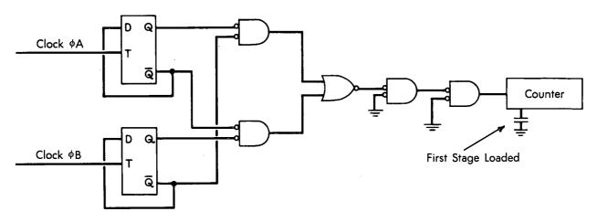
The "Sisyphus" experiment for a Pioneer probe required the operation of a binary counter at 4 MHz at low levels of power consumption, with bipolar TTL in the higher-speed portions of the circuits. Minimum weight requirements for the circuitry indicated the necessity of high-density packaging. As a result of high-density packaging, the logical gain-bandwith product of the devices used was significantly increased; this was attributed to short, low-capacity interconnections.
