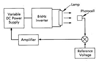
Wide-spectrum fluorescent lamps are to be used in this experiment, but since it is known that their luminous output decreases continuously, it is necessary to provide an illumination control system.
