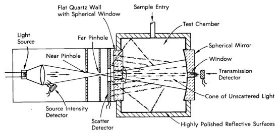
small particles is optimized because both scattered and transmitted illumination levels are detected by photodiodes. The light source, the optical system, and the test chamber are integrated into a single mechanical unit with an internal volume of 1.0 cm<sup>3</sup> and external dimensions 3.8 x 2.5 x 1.9 cm; the walls of the test chamber are highly polished.
