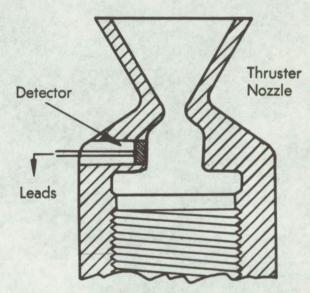
It has been shown that a small avalanche detector can sense radioactive gas leaking through a gas jet nozzle, but only marginally. On the other hand, if the detector area can be increased, the lower limit for sensing leak rates is lowered proportionally and quantitative measurements of leak rate can be made.
