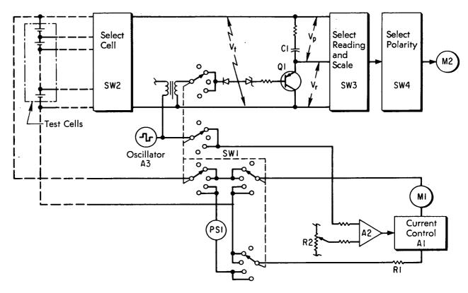
An improved Kordesch-Marko interrupter bridge circuit for measuring the IR-drop and IR-free voltage of electrochemical cells under load conditions has been developed and constructed. New features include the capability of varying the frequency of interruption in steps from 60 Hz to 2000 Hz, the extension of range to handle stacks of 10 or more cells in series, and the addition of operating modes to allow the instrument to serve as a steady DC
