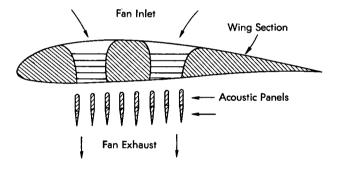
concept of using acoustic materials strategically located within or near noise sources appears to be straightforward and readily adaptable to situations outside of aircraft technology.
