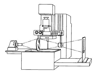
alignment. An electrode 12 to 15 cm in length and 1 mm in diameter can be easily straightened to a runout well within 0.050 to 0.075 mm.
