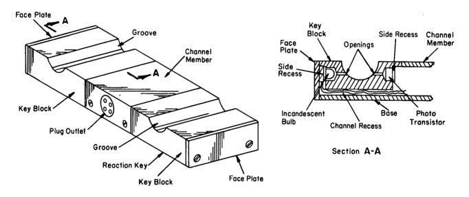
A new testing device measures the simple and disjunctive reaction time of a human subject to light stimuli. It consists of a reaction key, a logic card, panel mounted neon indicators, and interconnecting wiring. The logic circuitry indicates correct or incorrect responses and determines the reaction times with a maximum uncertainty of 56 microseconds. This includes all delays in the logic, light stimuli turn-on, and reaction key.
