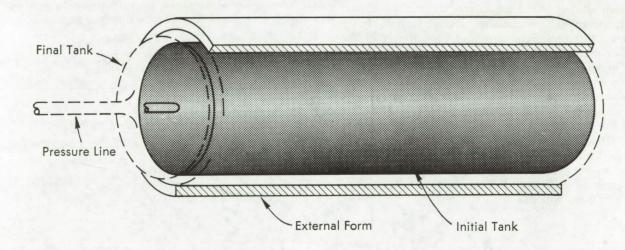
The need for reducing tank construction costs for the Space Shuttle was clearly evident from the beginning of the program, for it was realized that nearly one third of the direct cost per flight could be represented by the expendable hydrogen tanks unless their manufacture could be accomplished more cheaply. The results of a series of feasibility studies revealed that current manufacturing techniques or contemplated developments would not reduce costs significantly.
