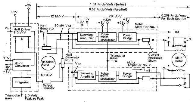
The motor control system consists of a Hall-effect generator/resolver and associated electronic amplifiers and switches. The system controls the power supplied to the motor's stator windings, causing the stator to produce a magnetic field that varies with the position of the resolver rotor. The resolver rotor is mechanically coupled to the main permanent-magnet rotor, and is aligned so that the stator field constantly
