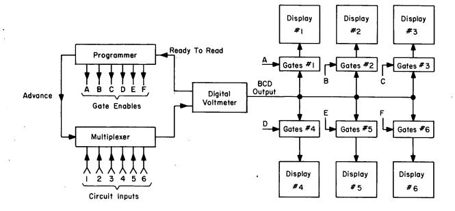
When designing and testing electronic circuits it is often desirable to measure several voltages and currents simultaneously. Digital voltmeters provide a rapid, accurate method of measuring electrical parameters and, when used with a multiplexer, provide the means of obtaining several simultaneous measurements.
