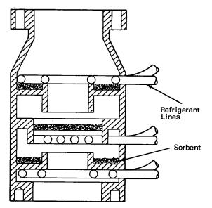
baffles connected in series with the sorbent traps, but these tandem combinations often reduce pumping speeds by a factor of two.
