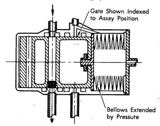
Gas Sampling Valve in Position after Gas Sample Delivery
