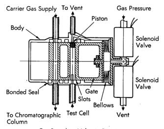
Gas Sampling Valve in Position prior to Gas Sample Delivery
