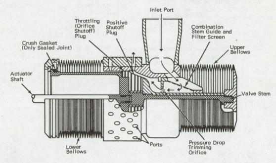
welded into the fuel lines. Seals or potential leak paths are minimized, and the valve operates with a short working stroke to provide maximum throttling sensitivity commensurate with good control. Individual injection orifices (not part of the valve), fed through tubing connected to the valve ports, provide essentially identical flow rates. Operation of the valve in this manner should ensure positive control of the injector hydraulic system while maintaining
