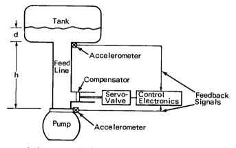
techniques employing standpipes, tuned pistons and accumulators could only reduce the amplitude of vibration-induced pressures, and required a knowledge of the system resonance, damping and transfer characteristics. The new technique has simplified the fluid system design and has eliminated the necessity for knowing the system response characteristics.
