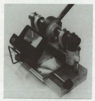
A precision die-punch will trim the conductors of FCC to a width of 0.040 in., adapting the cable for termination with a standard FCC plug which employs a window piece with 0.048 in. openings and a conductor spacer with 0.044 in. wide slots.
