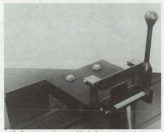
tool for preparing molded-plug terminations (see Note 1). It is necessary that the window piece be seated firmly against the cable insulation and that
